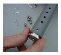
Install these one screw and washer in each end cap on the same side of the coil form. The other side will be used for securing the coil windings.
