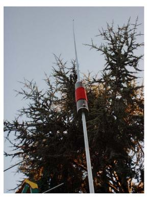
For operation, connect the radial wires or counterpoise to the ½" bolt in the center of the feed point using the supplied wing nut to secure the ring terminals on the radial wires. Deploy the radials around the base of the antenna as uniformly spaced as possible.
