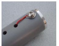
To allow adjusting the coil turns, attach this end as shown in the photo. This is temporary to allow removing turns if necessary to optimize the coil.
