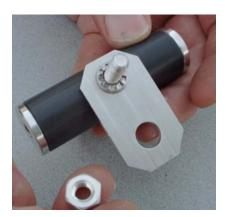
Using the ¼ -20 x 1.5" bolt, lock washer and nut, attach the BNC mounting plate to the feed point insulator PVC tube by inserting the bolt through the PVC tube and then through the aluminum bnc mounting plate.
