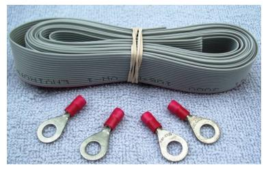
Parts: 16-conductor ribbon cable 4 -1/4" ring terminals
