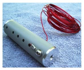
Attach the ring terminal on the end of the wire to the end cap of the coil with a screw and lock washer.
