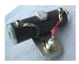
Once the BNC is securely installed, use the sections of green and red wire to connect from the BNC to the crimp terminals. The red wire goes the center terminal of the BNC. The red wire will indicate the antenna end of the feed point.
