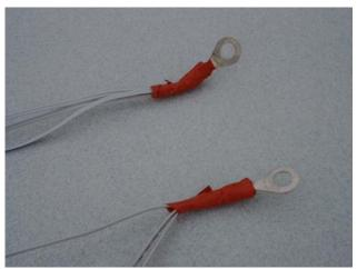
Crimp the terminal and use electrical tape or heat shrink tubing to strain relief the connection. Separate the sets of 4 wires into two wire sets from the end up to the strain relief on the ring terminal. This will form 2 radial wires connected to each ring terminal. Each radial will have 2 parallel conductors.
