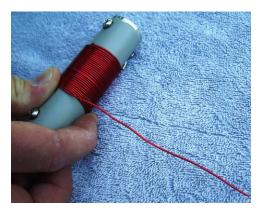
Begin winding the coil by turning the form while feeding the wire onto it. Using the thumb and forefinger will work to guide the wire. Wind the specified number of turns on the coil. A turn counts each time the wire loops completely around the coil from the starting point. If in doubt, put on extra turns as it is easier to remove an extra turn than to rewind the coil. When finished, cut off the excess wire leaving about 6". This will allow the end to be passed back through the coil form.
