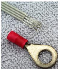
Strip the ends of the wires back a half-inch or so, and twist them together.
