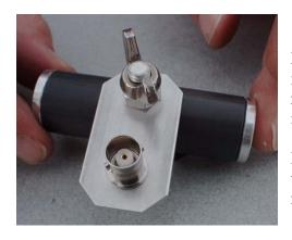
Mount the BNC in the plate and secure using its nut. The BNC connectors may be supplied with a red rubber gasket that should be removed before installation
