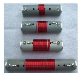
This is what the coils will look like when completed. The instructions below will step through the process of assembling and winding the coils for your PAC-12.
