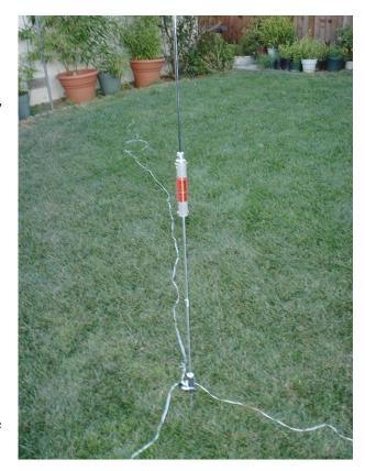
Connect the whip to the other end of the coil by screwing the adapter into the threaded opening in the coil. This completes assembly of the antenna.
