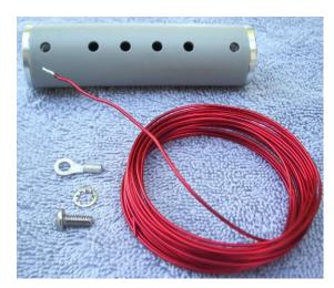
First, tin the end of the enamel wire by heating with a blob of solder. Feed extra solder in as necessary and you will see the enamel begin to peel off and the solder will coat the bare end. Tin approximately 0.25 to 0.5" of the wire to prepare it for connection at the crimp terminal later.
