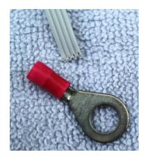
First, separate the 16-conductor ribbon cable into 4-conductor sections giving a total of 4 sections of 4 wires each.. .
